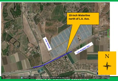
Install approximately 5,000 lf of 10-inch water line and appurtenant work to improve operational flexibility in the system per Master Plan.
