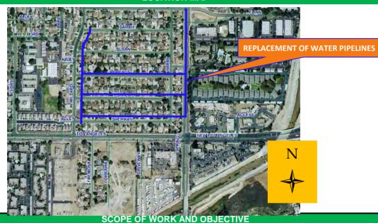
Installation of approximately 5,600 LF of 8-inch water line to replace the substandard and aging 4-inch lines with 8-inch lines per master plan udate,
