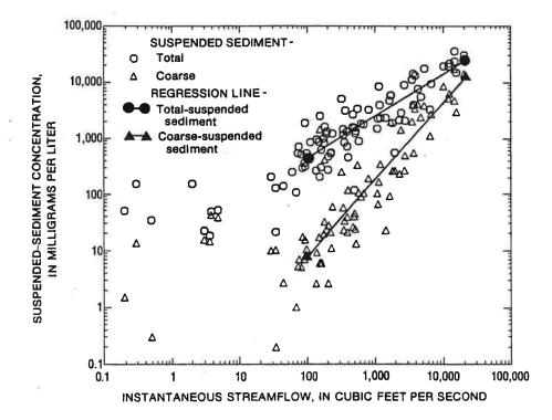
FIGURE 3.--Concentration curves for total-suspended and coarse-suspended sediment, Ventura River near Ventura (11118500).
