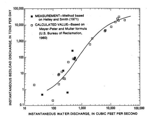
FIGURE 2.--Bedload-transport curve, Ventura River near Ventura (11118500).
